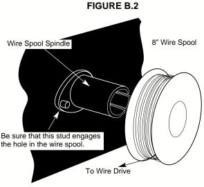
Wire Spool must be pushed all the way on the spindle so that the spindle's tab will hold it in place. The Wire Spool will rotate clockwise when wire is dereeled.
